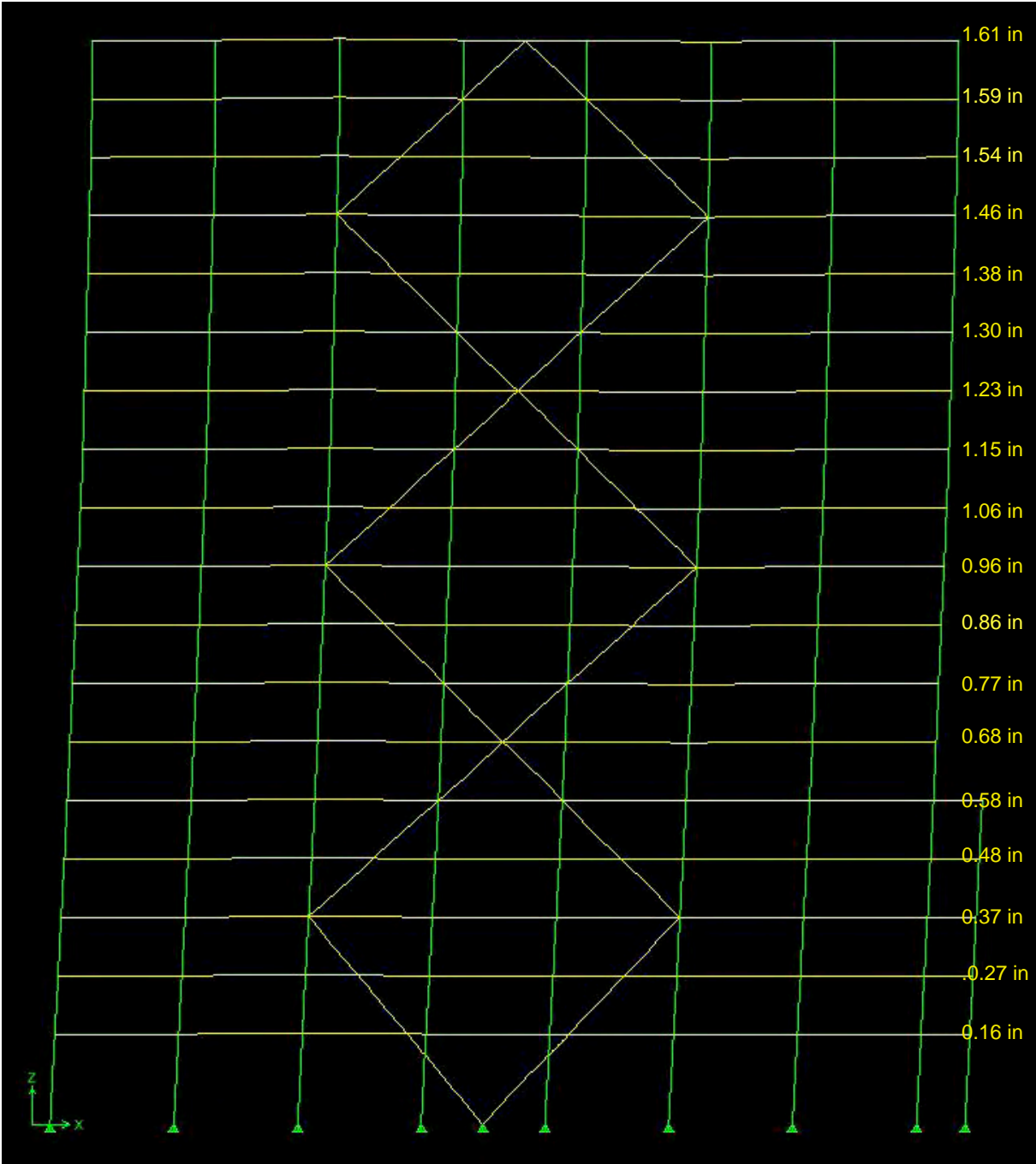
Deflections due to Response spectrum analysis in East-West direction
